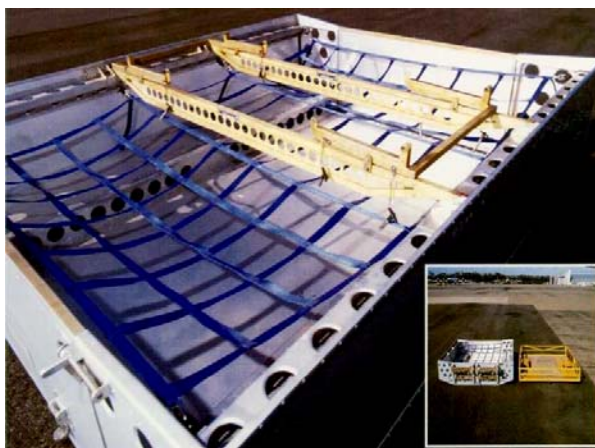
AFTS High Capacity Cargo Pannier for Orion P-3 aircraft for carriage of 2,000 lb cargo in bomb bay
