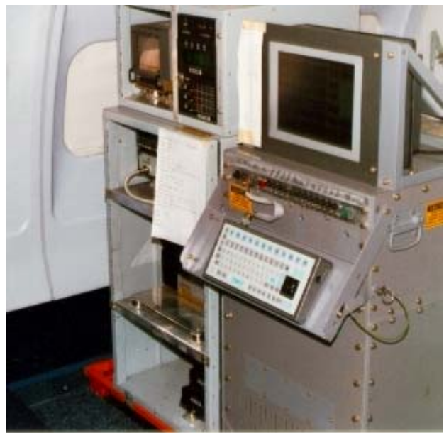
AFTS Data Acquisition System (ADAS MkII) installed in RAAF B-707 for flight test data trials.
