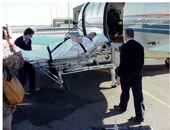
AFTS Stretcher Loading Device (SLD) and Aeromedical Stretcher (752TA) on PC-XII aircraft
